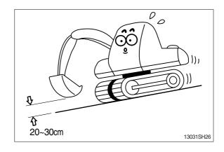
Steering of the machine while traveling on a slope is dangerous.
