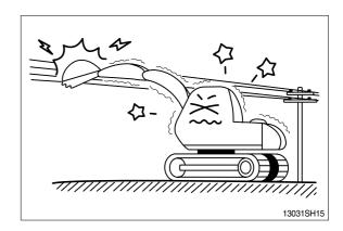
If the machine touches the electric power lines, keep sitting on the operator's seat and make sure the personnel on the ground not to touch the machine until turning off the electric current. Jump off the machine without contacting the machine when you need to get off.
